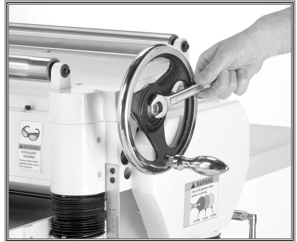
Figure 6. Installing handwheel on shaft.
